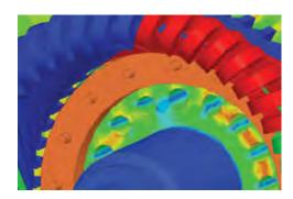
Engineers at WEG Equipamentos Elétricos S.A., Brazil, used Maxwell in a multiphysics simulation to optimize the trade-off between fan losses and electromagnetic performance in its new line of electric motors.
