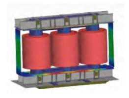
Pennsylvania Transformer Technology, Inc. performed multiphysics simulations using Maxwell, Ansys Mechanical and Ansys CFD to design next-generation transformers for the utility power industry.
