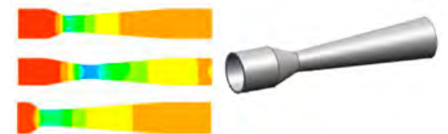
When optimizing the air intake for an FSAE car, the University of Waterloo Formula Motorsports team used DesignXplorer to quickly and efficiently investigate design impact on overall performance, eliminating the need for multiple prototype cycles.
